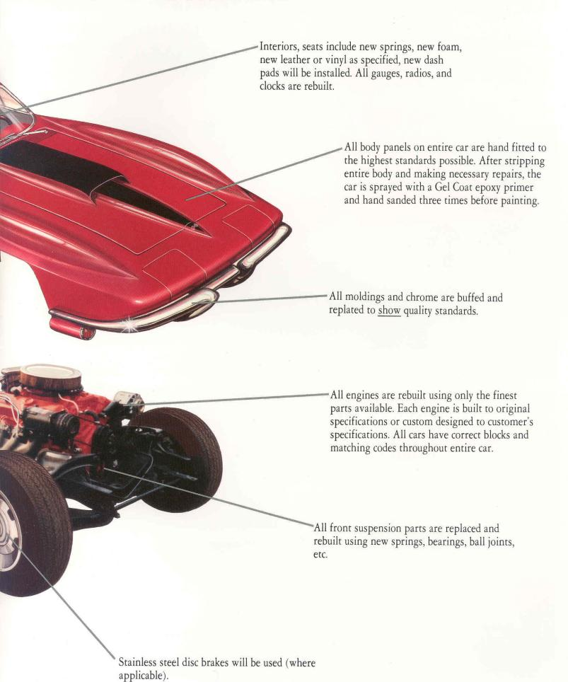
OVER 500 HOURS ARE REQUIRED FOR A CORVETTE TO BE REMAN-UFACTURED TO OUR EXACTING STANDARDS. OUR CORVETTES
